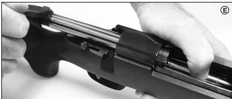
Closing the bolt over the loaded magazine
